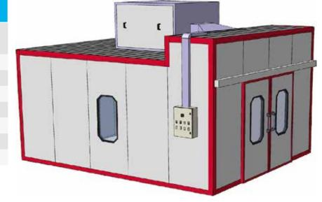
This type of system is suitable for the drying of freshly painted products in a dust free environment and with consistency in temperature. It is built with sandwich panels. The air flow for drying the products is created by a pressurized and extraction units.
