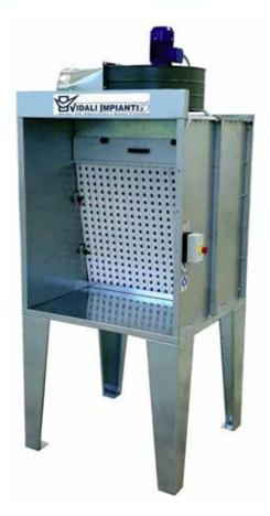
This type of painting booth is suitable for suctioning and demolishing the pigments and fumes emitted from paint-spay made with synthetic solvents, organic and water. The removal of the pigments and fumes occurs with a suctioning wall of cardboard inertial and a second filtration with "Paint-Stop" filter drawers. It is used mainly for the painting of small objects, for the testing of paint for laboratories. This booth is built with modular panels of galvanized press-folded sheet-iron.
