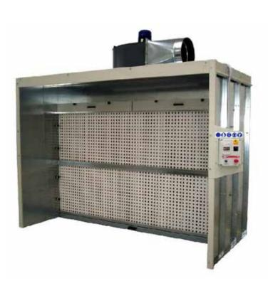
This type of painting booth is suitable for suctioning and demolishing the pigments and fumes emitted from paint-spay made with synthetic solvents, organic and water. The removal of the pigments and fumes occurs with a suctioning wall of cardboard inertial, a second filtration with "Paint-Stop" acrylic filter and a third filtration with active carbon. The paint booth is built with modular panels of galvanized press-folded sheet-iron.
