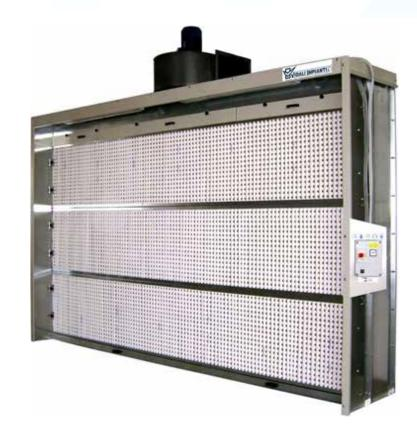
This type of painting booth is suitable for suctioning and demolishing the pigments and fumes emitted from paint-spay made with synthetic solvents, organic and water. The removal of the pigments and fumes occurs with a suctioning wall of cardboard inertial and a second filtration with "Paint-Stop" filter drawers. It is utilized for painting elements that are over-sized. The paint booth is built with modular panels of galvanized press-folded sheet-iron.
