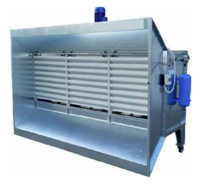
This type of booth is indicated for the suctioning and removal of dust from sanding. It is built with galvanized press-folded sheet iron. The main feature of this booth is the filtration of dust through aluminized polyester antistatic cartridges. The booth is equipped with a cleaning system of the cartridges with jets of compressed air. The dust is deposited in 2 removable trays.
