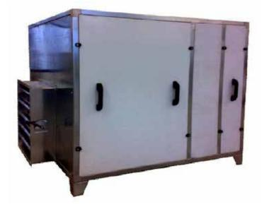
The pressurized group is constructed with a load- bearing frame and insulated perimeter panels with interposition of glass wool. Drive train exhaust fan with double inlet transmission belt. Intake acrylic filter. Complete with damper adjustment.
