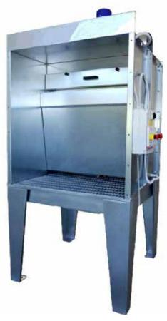
This type of painting booth is suitable for suctioning and demolishing the pigments and fumes emitted from paint-spay made with synthetic solvents, organic and water. The removal of the pigments and fumes occurs with a frontal veil of water and with "Paint-Stop" filter. It is used mainly for the painting of small objects, for the testing of paint for laboratories. This booth is built with modular panels of galvanized press-folded sheetiron.
