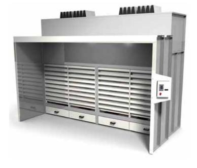
This type of booth is indicated for the suctioning and removal of dust from sanding. It is built with galvanized press-folded sheet iron. The main feature of this booth is the filtration of dust through aluminized polyester antistatic cartridges. The booth is equipped with a timed self cleaning system of the cartridges with jets of compressed air. The dust jets are deposited in removable trays.
