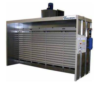
This type of booth is indicated for the suctioning and removal of dust from sanding. It is built with galvanized press-folded sheet iron. The main feature of this booth is the filtration of dust through aluminized polyester antistatic cartridges. The booth is equipped with a cleaning system of the cartridges with jets of compressed air. The dust jets are deposited in removable trays.
