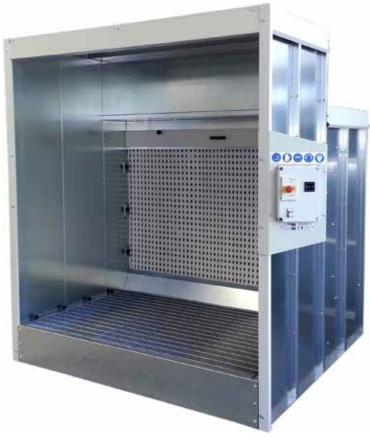
This type of painting booth is suitable for suctioning and demolishing the pigments and fumes emitted from paint spray made with synthetic solvents, organic water. The removal of the pigments and fumes occurs with a suctioning wall of cardboard inertial and a second filtration with "Paint-Stop" filters drawers. The paint booth is built with modular panels of galvanized press folded sheet iron.
