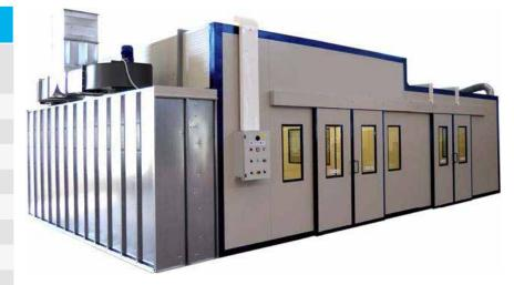
This type of pressurized system is indicated to perform the painting by creating a dust free environment. It can be combined with a dry painting booth or water painting booth(not included in price). It is built with pre painted sandwich panels. The characteristic of this system is the double airflow in the area of coating and drying. The air is blow through a prefilter and a large filter.
