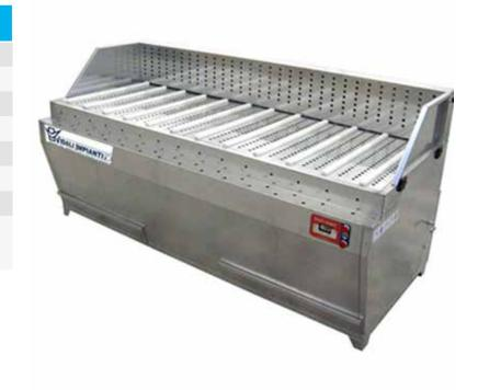
This type of bench is indicated for the suctioning and removal of dust from sanding. It is built with galvanized press-folded sheet iron. The main feature of this bench is the filtration of dust through aluminized polyester antistatic cartridges. The bench is equipped with a cleaning system of the cartridges with jets of compressed air. The dust is deposited in 2 removable trays. The outgoing air is further filtered through acrylic fiber cells.
