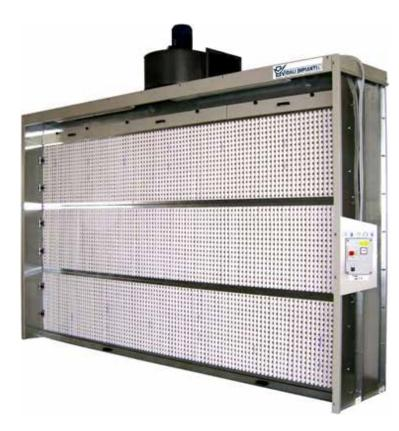
This type of painting booth is suitable for suctioning and demolishing the pigments and fumes emitted from paint spray made with synthetic solvents, organic water. The removal of the pigments and fumes occurs with a suctioning wall of cardboard inertial and a second filtration with "Paint-Stop" filters drawers. The paint booth is built with modular panels of galvanized press folded sheet iron.
