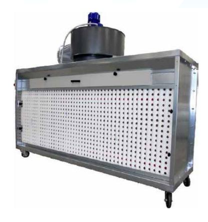
This type of painting booth is suitable for suctioning and demolishing the pigments and fumes emitted from paint-spay made with synthetic solvents, organic and water. It is built with modular panels of galvanized pressfolded sheet-iron. The main features of these booths are their small dimensions and the possibility of easy transfer. This booth utilizes a suctioning wall of cardboard inertial and a second filtration with "Paint-Stop" filter drawers.
