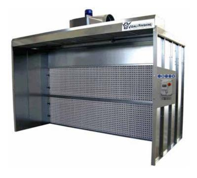
This type of painting booth is suitable for suctioning and demolishing the pigments and fumes emitted from paint spray made with synthetic solvents, organic water. The removal of the pigments and fumes occurs with a suctioning wall of cardboard inertial and a second filtration with "Paint-Stop" filters drawers. The paint booth is built with modular panels of galvanized press folded sheet iron.
