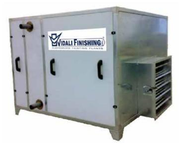
The pressurized group is constructed with a load-bearing frame and insulated perimeter panels with interposition of glass wool. Drive train exhaust fan with double inlet transmission belt. Intake acrylic filter. Radiant battery (differential thermal 25°). Complete with damper adjustment.
